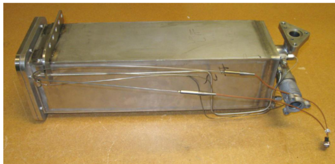
hot reformat desulfurizer
